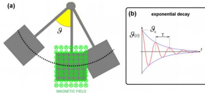
(a) A metallic pendulum oscillates inside and outside the magnetic field region generated by a permanent magnet. (b) The oscillation amplitude decays exponentially with time as described by Eq.
